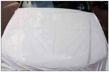
By breaking up the hood into four triangles, it enabled me to wrap cars more efficiently by myself.
