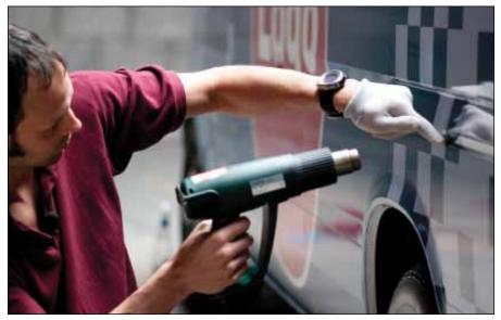
I use application gloves to apply the film to recessed areas to help work in otherwise tricky sections.
