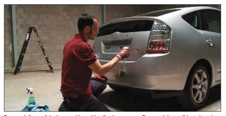
Be especially careful when working with adhesive remover. Because it is an oil-based product, any residual drips that go un-cleaned will result in poor adhesion of the wrap.
