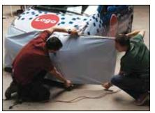
To avoid bunching on bumpers, have one installer hold the film away from the corner while other installer warms the film with a heat gun. Once the film is warm, one installer can pull the film around the corner horizontally while the other pulls the film away from the center at a 45-degree angle.
