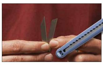
The knife you use for wraps installation can affect the quality of your installation. For vehicle graphic installations, it's best to use a multicartridge knife loaded with blades that feature a 30-degree angle.
