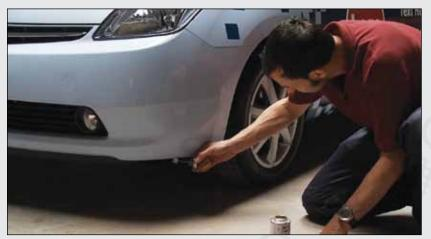
Using edge sealer on the edges of wheel wells and underneath the bumper will help prevent winter road salt and chemicals from reacting with adhesive, which leads to peeling.
