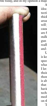
A thick buffer may seem like a good idea because of the perceived extra protective qualities, but a squeegee with a thick buffer is only really effective on flat areas. On any kind of curve, a thick buffer will push the film, and that will quickly cause the film to bunch up. Since vehicles are full of curves, this means that an installer is forced to resort to using a heat gun to soften out bunched-up film. This really slows down the installation process and often leads to overstretching.
