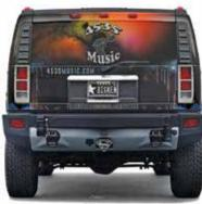
Image C: This Hummer design does not follow the threeinch rule. Text was placed too close to many of the vehicle's installation hot spots.
