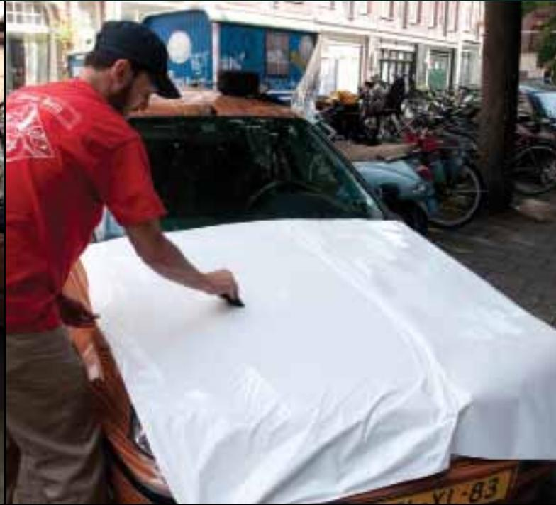
When I set my hinge in the middle of the hood, instead of making long, horizontal squeegee strokes toward the side, I broke half of the panel up into two triangles. I did this by making a squeegee stroke to the side from the vertical hinge in the middle.
