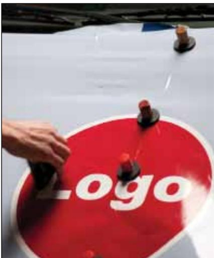
**I use magnets with handles to hold the panels on the vehicle.**
