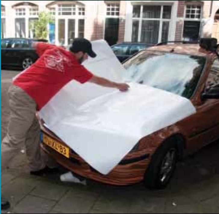
Wrapping vehicles by myself means that I get all the profit from an install, but it also means that I have to find ways to apply large, awkward panels by myself.
