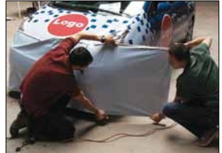
To avoid bunching on bumpers, have one installer hold the film away from the corner while other installer warms the film with a heat gun. Once the film is warm, one installer can pull the film around the corner horizontally while the other pulls the film away from the center at a 45-degree angle.
