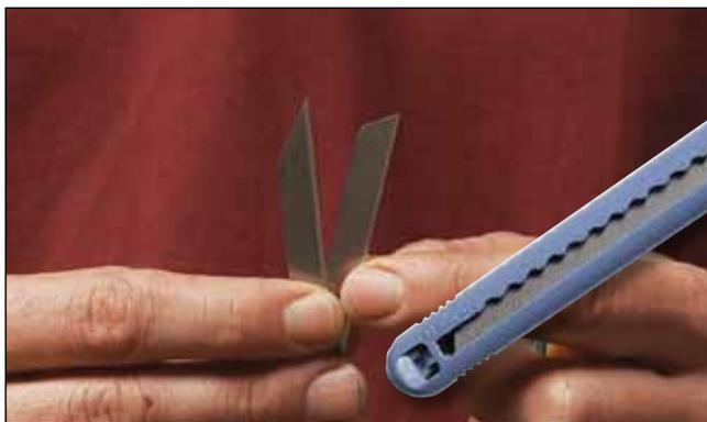
The knife you use for wraps installation can affect the quality of your installation. For vehicle graphic installations, it's best to use a multi-cartridge knife loaded with blades that feature a 30-degree angle.
