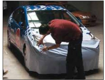
Bunched film on the corners of bumpers often results in overstretching and frustration. The key to these corners on the bumper is to set the film up properly.
