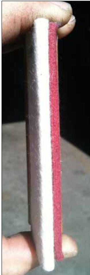
A thick buffer may seem like a good idea because of the perceived extra protective qualities, but a squeegee with a thick buffer is only really effective on flat areas. On any kind of curve, a thick buffer will push the film, and that will quickly cause the film to bunch up. Since vehicles are full of curves, this means that an installer is forced to resort to using a heat gun to soften out bunched-up film. This really slows down the installation process and often leads to overstretching.
