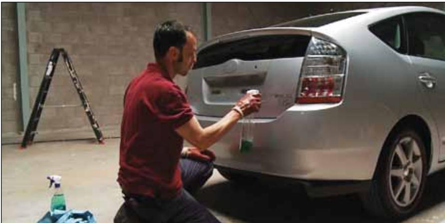
Be especially careful when working with adhesive remover. Because it is an oil-based product, any residual drips that go un-cleaned will result in poor adhesion of the wrap.
